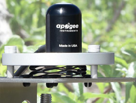
Measure photosynthetically active radiation (PAR) in  $\mu\text{mol m}^{-2} \text{s}^{-1}$
