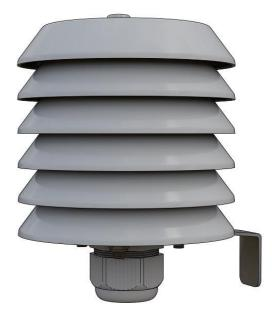
Another benefit of the Meteobot® radiation shield is that it provides for much more sensitive readings when the temperature changes. This is because the construction is well-ventilated and the polypropylene material itself quickly warms up or cools down during temperature fluctuations. This is a considerable advantage over traditional wooden radiation shields, which are "temperature-inert" and can typically lead to 1 - 1.5°C of "temperature lag".
